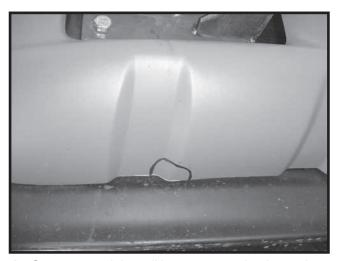
**6b.** On some models, pull bumper cover back to gain access to rear pull pod bolt, or notch out bumper cover according to picture to install bolt.
